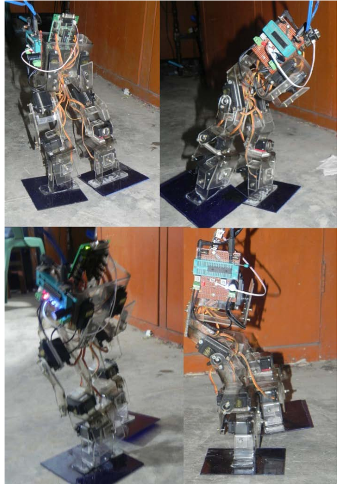
Fig 4. walking steps of bipedal robot
